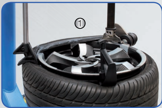
(1) Two help-arms for more efficiency (2) Powerful air jets in all clamping jaws (3) Large clamping range (4) Powerful bead breaker
